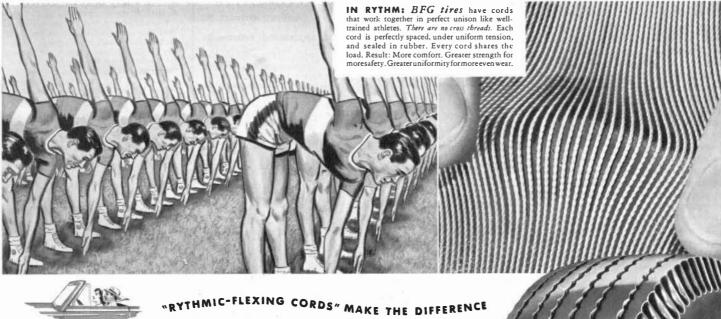
Inside every tire are thousands of cords that flex constantly—over bumps and chuck-holes, and every time the tire revolves. In most tires these cords are loosely tied together by cross threads, which keep the cords from flexing evenly. As a result, some cords carry too much load, others work too little.
